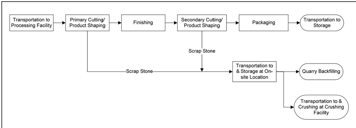
Figure 2. Process flow diagram for processing operations.
