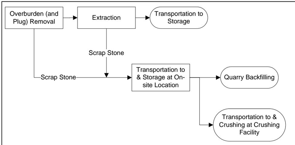
**Figure 1. Process flow diagram for quarrying operations.**
